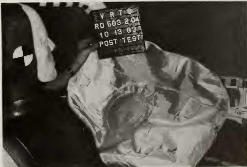
Face Impact Area On Airbag Test 4
